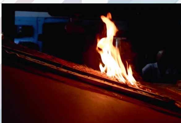
Photo of a flame when a layer of pine needles burns on an inclined (15° — left picture) and horizontal surface (right picture), side view.
