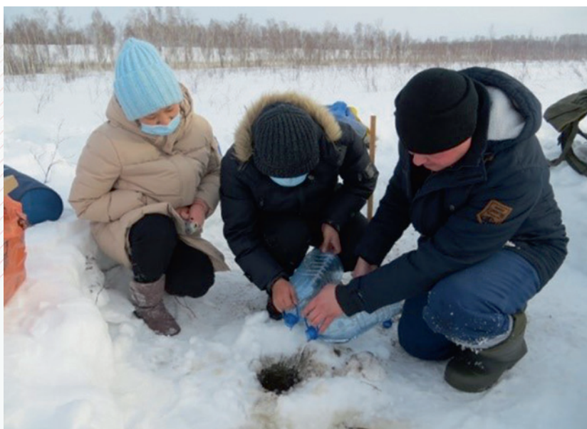
Release of NaCl solution on the surface of the Ob bog (the hole is made in the fringe) March 19, 2021; Associate Professor of TPU Ivanov A.Yu, graduate students of TPU Zhou Dan and Yang Heng
