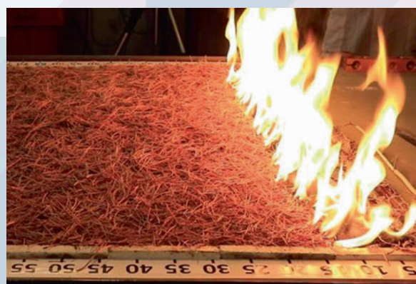
Photo of a flame when a layer of pine needles burns on an inclined (15° — left picture) and horizontal surface (right picture), side view.
